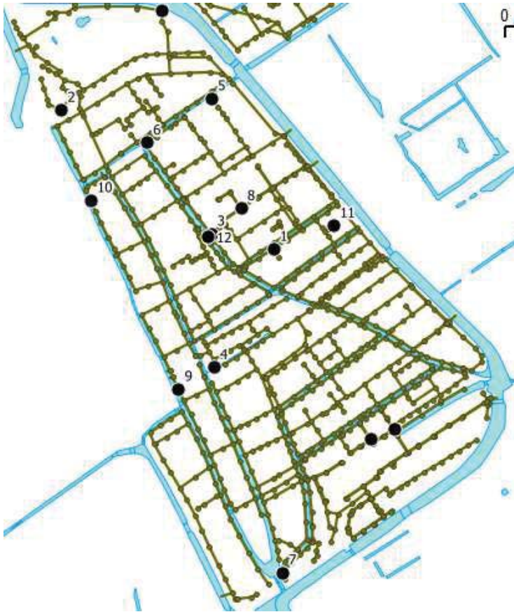
Figure 48: Spatial distribution of the 12 sensors derived from the optimisation algorithm
